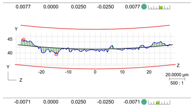
Fig. 24 Minimum error of tooth line
