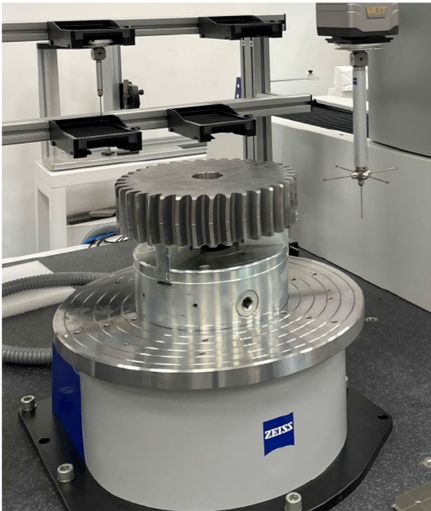
Fig. 20 Detection of gear surface data
