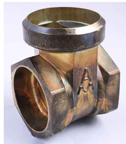
Fig. 9 Valve body forged by CuZn39Pb2 continuous casting workpiece with a hexagonal cross-section
