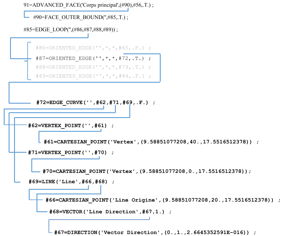
Fig. 17 Diagram for determining the linear curve for the generation by revolution of a simple cylinder
