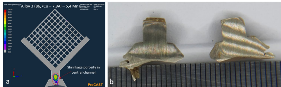
Fig. 19 a Section of the virtual casting of alloy 3 predicting a porosity region. b Section of the real casting showing no visual defects
