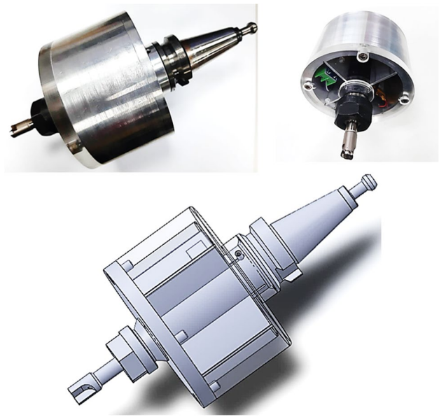
Fig. 8 On-line cutting temperature measuring tool holder
