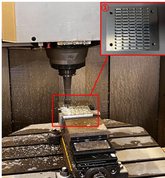
Fig. 10 Milling experiments (wet cutting) carried out on a Mikron vertical five-axis machining center. (①: Workpiece with the machined features.)
