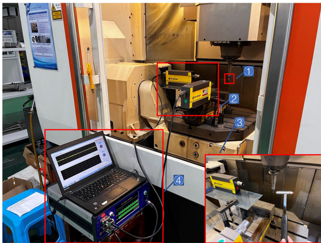
Fig. 6 Experimental configuration of the non-contact vibration measurement. (①: Milling cutter; ②: Vertically arranged Doppler vibrometers; ③: Hammer vibration test; ④: Data acquisition system.)
