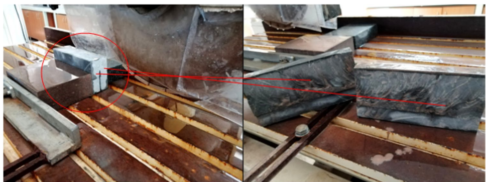
Fig. 7 Separation of the workpieces with a circular diamond saw
