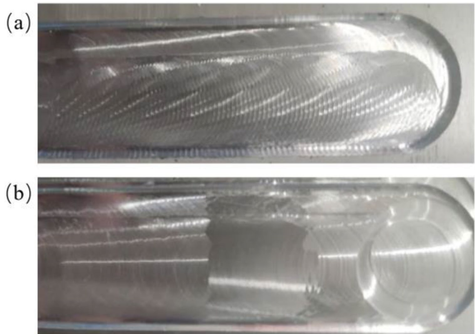
Fig. 11 Experimental surface characteristic: a surface characteristic after test no. 5 and b surface characteristic after stable milling
