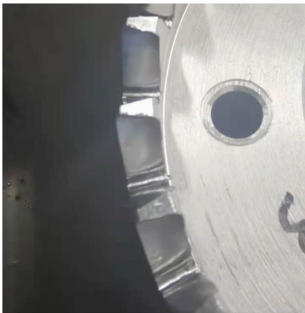
Fig. 10 Face gear based on five-axis side milling
