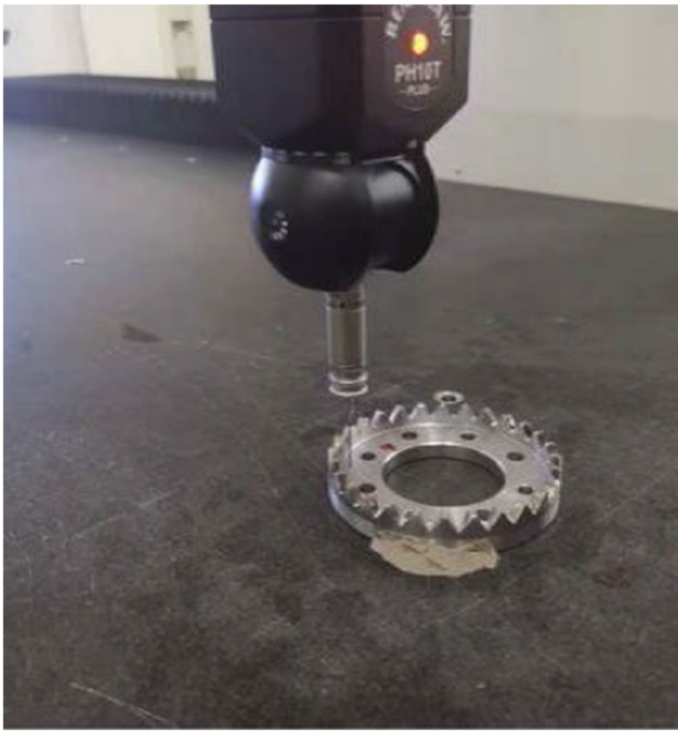
Fig. 17 Machining error measuring process of the face gear
