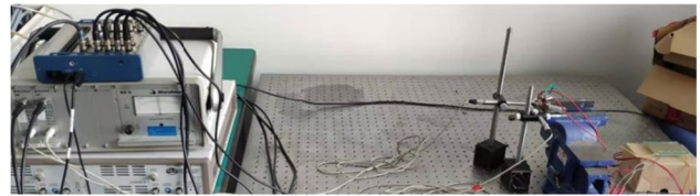
Fig. 4 Acquisition and analysis of electrical signal and displacement signal of ultrasonic vibration device
