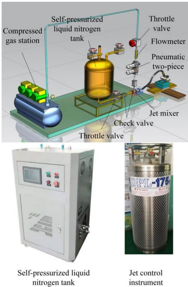
Fig. 1 Low-temperature jet cooling system
