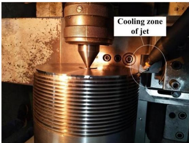
Fig. 3 Orthogonal turning experiment at low temperature
