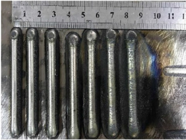
Fig. 10 Results of single-channel liner cladding experiment under different powers [55]
