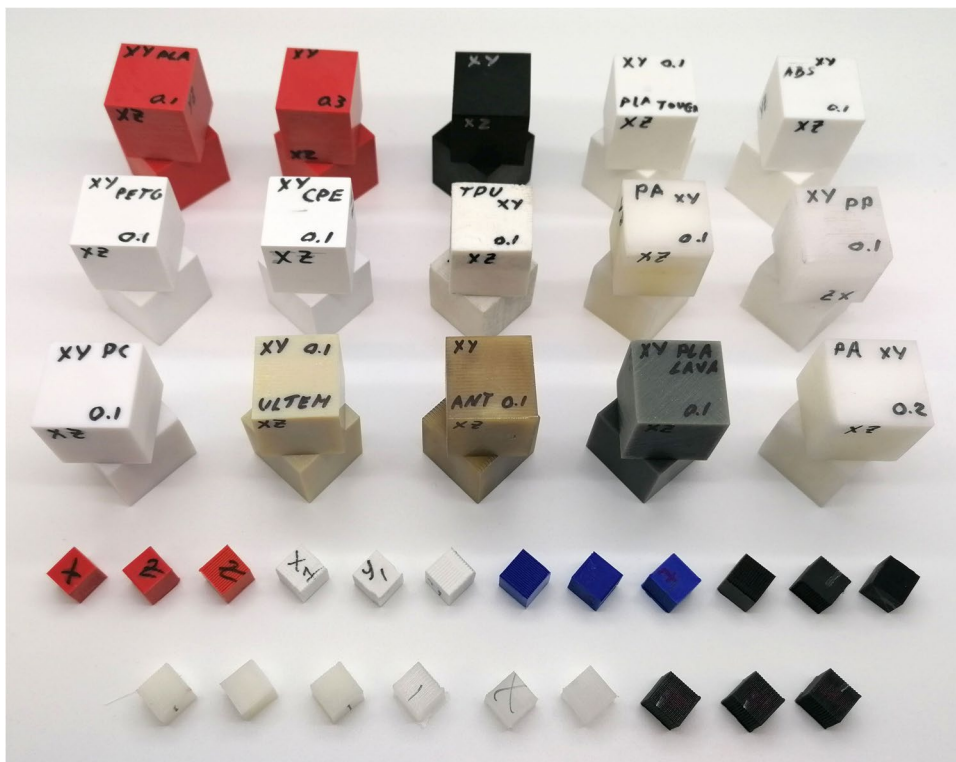
Fig. 1 Example of the investigated samples. Big cubic samples with dimensions 25×25×25 mm for determination of the thermal conductivity, and samples with sizes 10×10×10 mm for evaluation of CLTE and ITS
