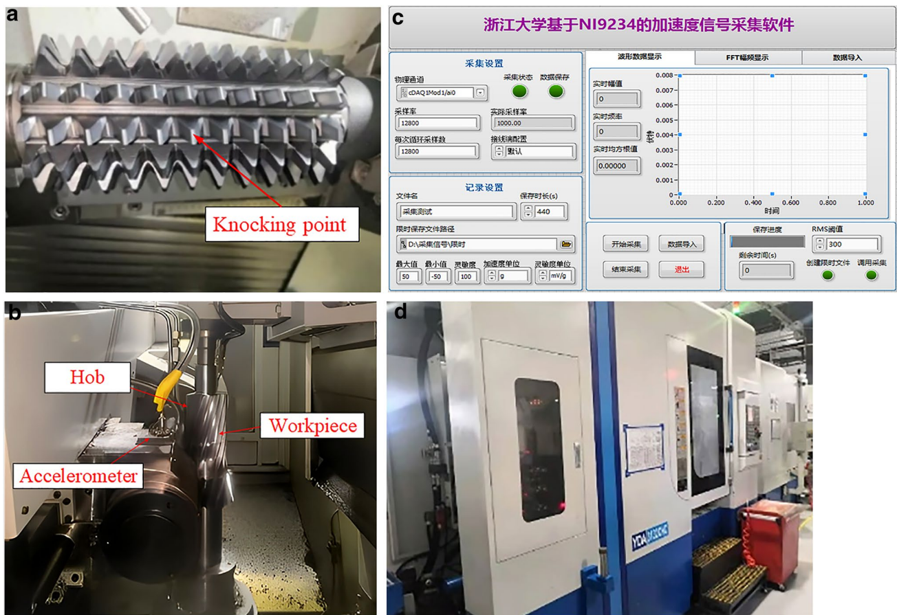
Fig. 10 Experimental equipment. a Hob. b The experimental platform for hobbing. c Data acquisition system. d Hobbing machine
