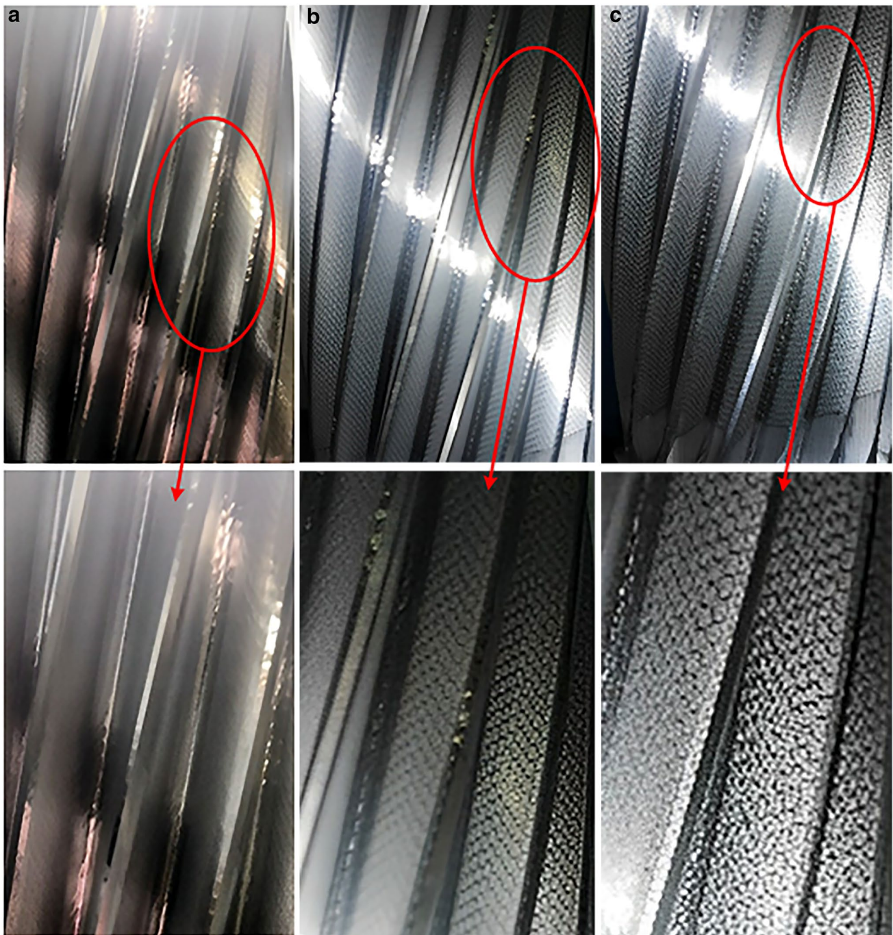
Fig. 14 Gears machined by hob in different wear states. a Initial wear. b Normal wear. c Severe wear
