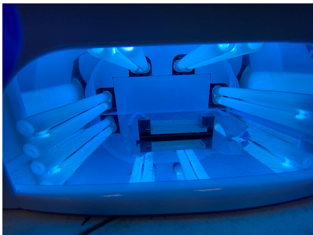
Fig. 6 NOA88 optical adhesive curing under UVA irradiation
