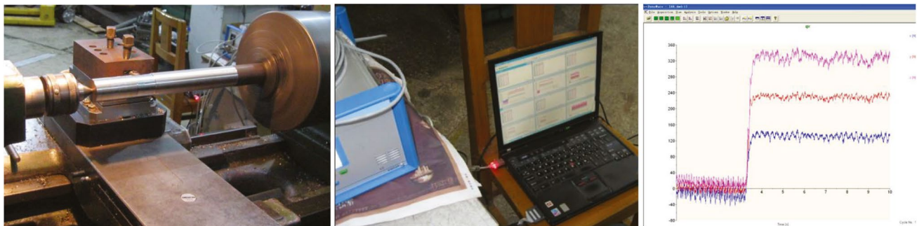
Fig. 12 The experiments of cutting forces in cylindrical turning of 304 stainless steel
