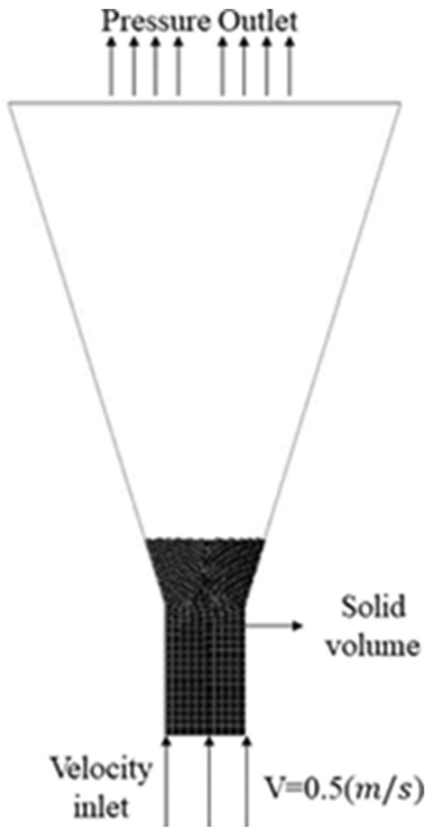
Fig. 3 Simplified model of abrasive pool
