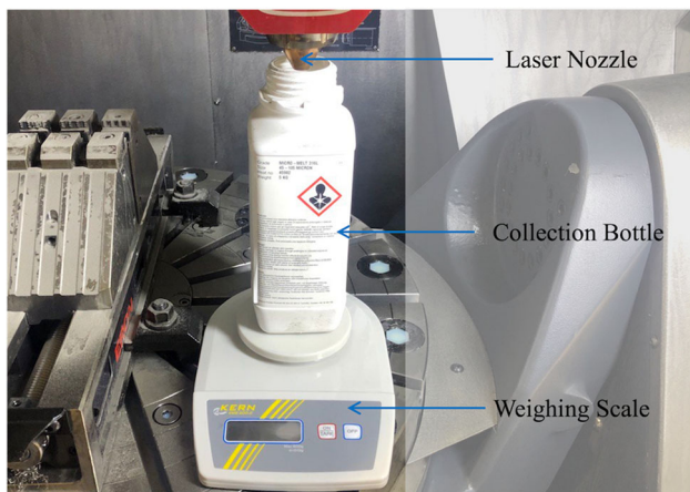
Fig. 2 Powder flow rate measurement setup with a digital weighing scale. A camera was used to record the weight increment over a duration of 1 min. For each voltage input, measurements were conducted thrice to obtain an average powder flow rate output
