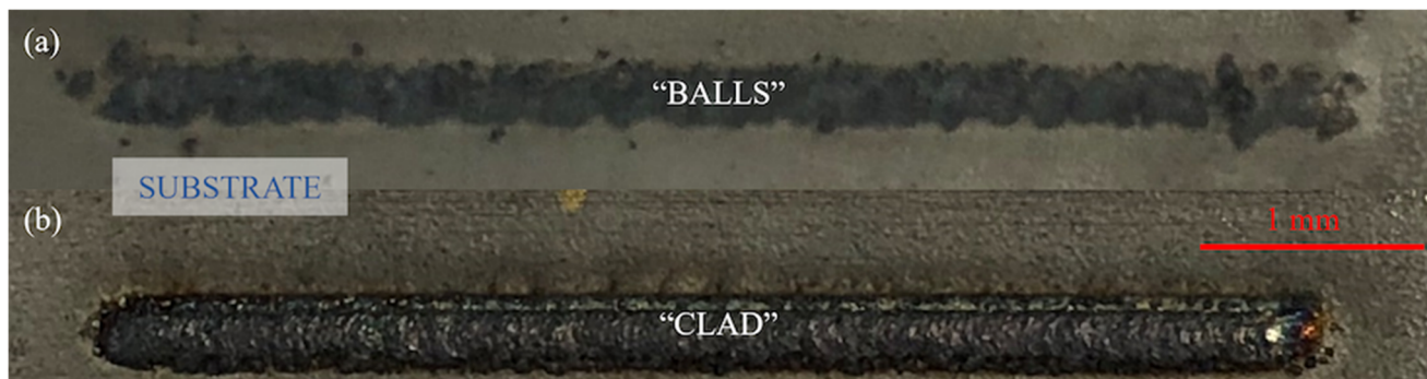
Fig. 5 Example of (a) a poorly bonded melt track and (b) a desirable clad
