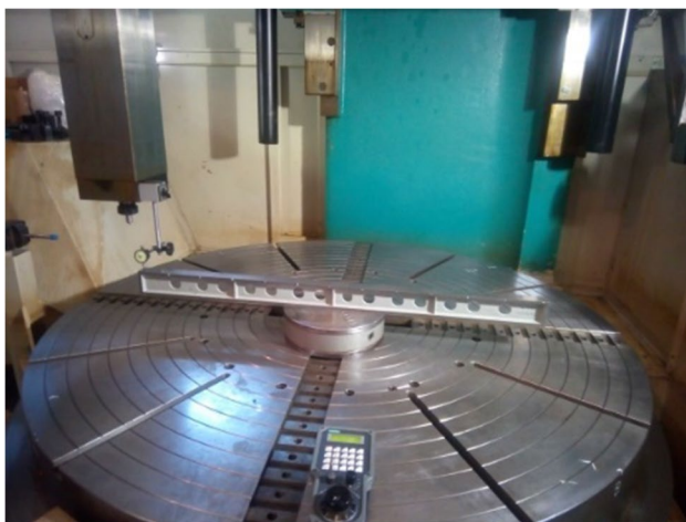
Fig. 12 Straightness measurements by hand tools
