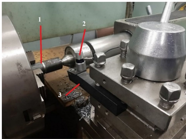
Fig. 5 Experimental set-up for vibration measurement, including 1, workpiece; 2, accelerometer KD-35; and 3, cutting tool
