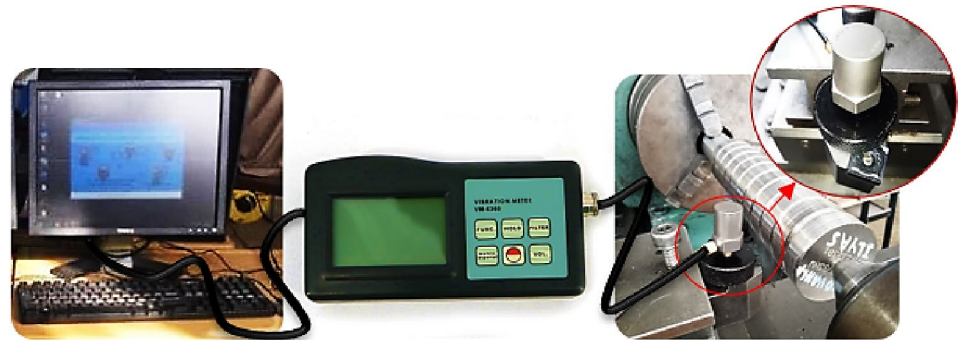
b). Vibrometer, VM 6360 Digital Vibration Tester + Accelerator with running software.
