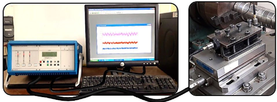
c). Dynamometer (KISTLER 9257 B) with kistler signal amplifiers, acquisition board and dynoware measurement program.
