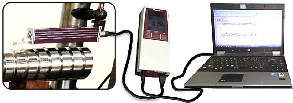
a). Mitutoyo SurfTest SJ-210 2D roughness tester with runtime software.
