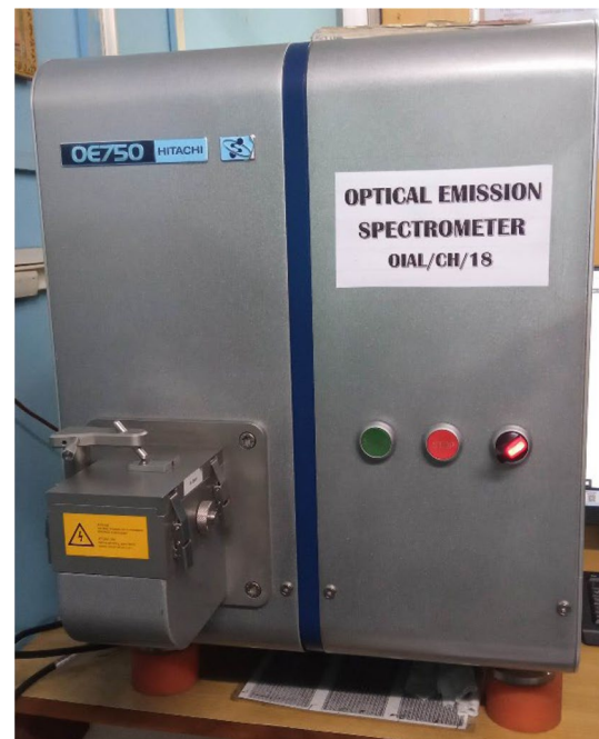
Fig. 1 Chemical analysis-optical emission spectrometer apparatus
