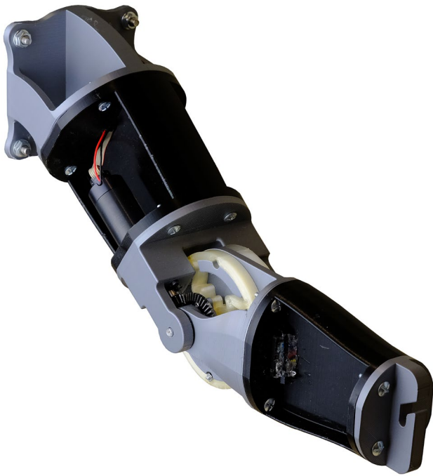
Fig. 1 Physical prototype of the variable stiffness elbow joint
