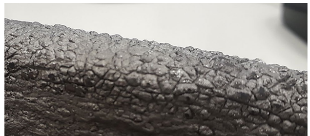
Fig. 8 Surface of a forged workpiece at the top of the wing
