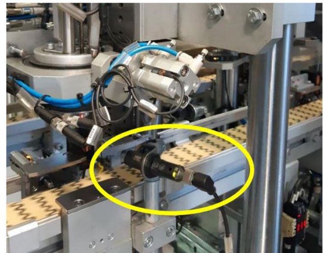
Fig. 11 Proximity sensor used as a stopper to limit buffer capacity on the linear rails
