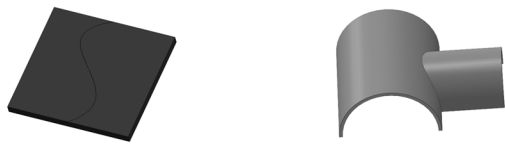
(a) The workpiece with S-shape weld seam (b) The workpiece with saddle-shape weld seam
