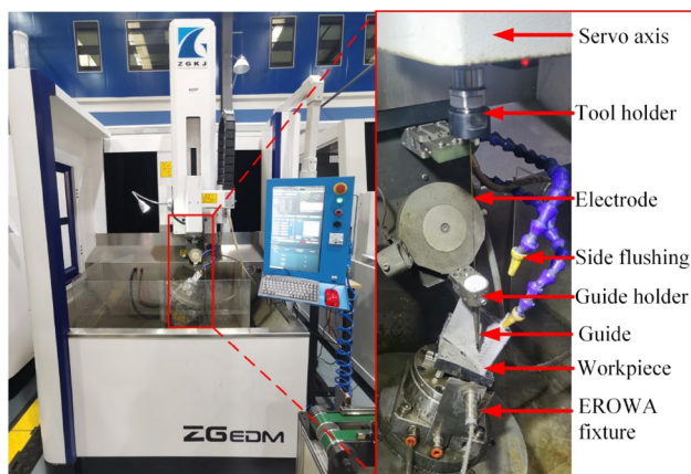
Fig. 2 The fast ED-drilling and milling machine
