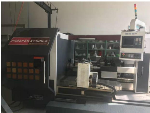
Fig. 6 PS-CNCSXY600-5 spinning machine
