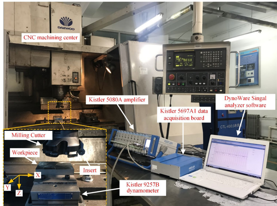
Fig. 2 Face milling experiments setup
