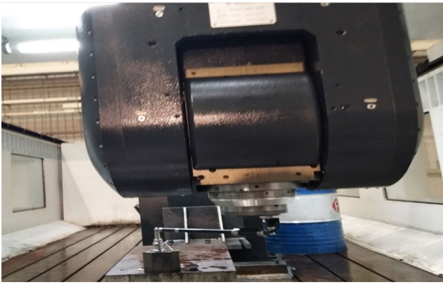
Fig. 4 The measurement scene of five PDGEs of C-axis
