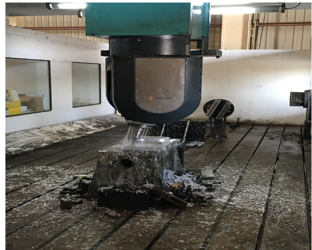
Fig. 7 The machining scene of S-shaped specimen
