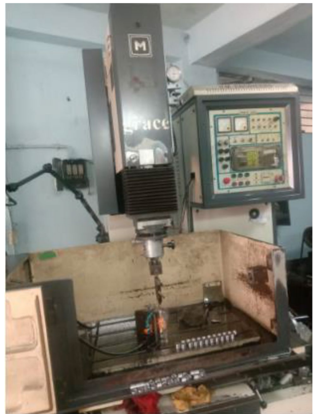
Fig. 4 Machining process of PM-EDM
