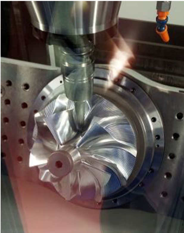
Fig. 16 Machining process of the impeller
