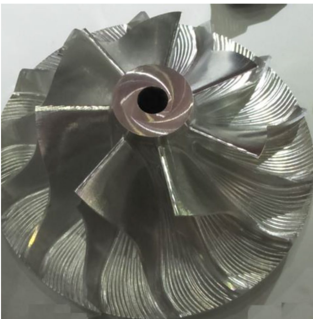
Fig. 17 Impeller with S-curve method
