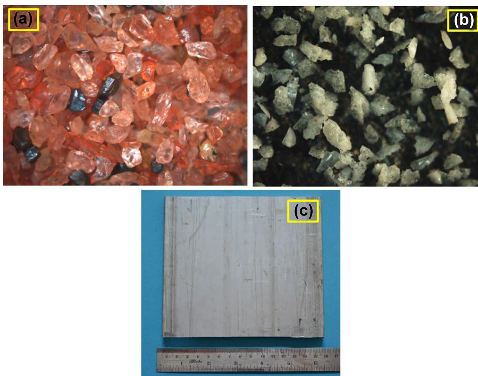
Fig. 3 Abrasive particle and workpiece material, (a) Garnet, (b) EIR particle, and (c) Aluminium target
