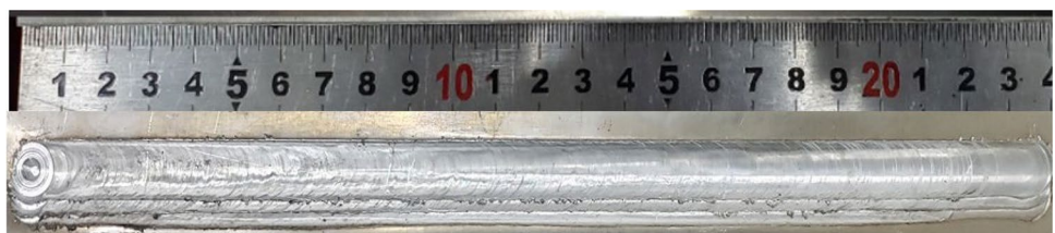
Fig. 7 Macromorphology of the foam precursor with welding spacing of 3 mm
