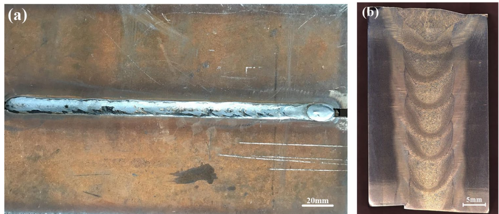
Fig. 5 Cross-section of the formed weld with CWW NG-GMAW. (a) Weld shape. (b) Cross-section of the weld seam
