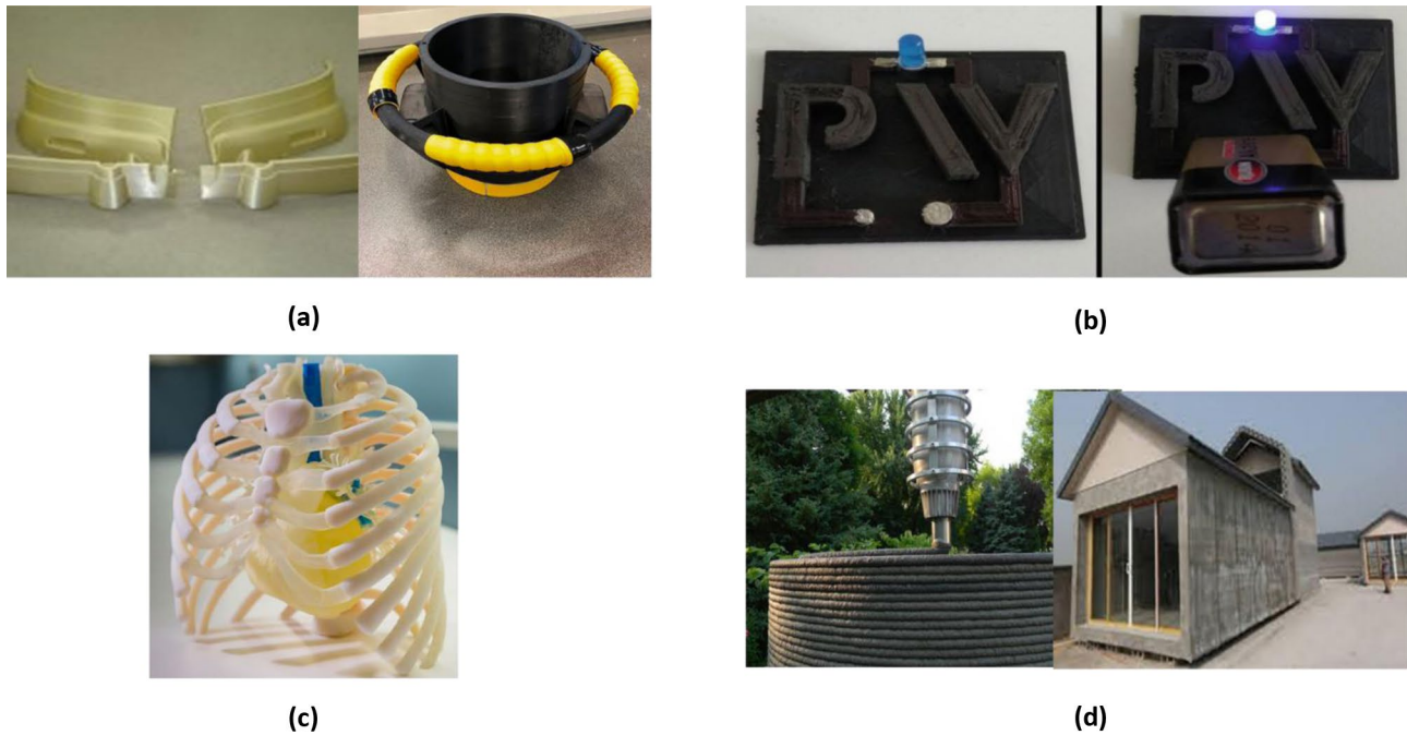
Fig. 15 a Evekotor aircraft components and FDM printed duct adapter [290]. b FDM-printed electric circuit with LED [291]. c FDM-printed Ribcage [292]. d FDM concrete printing process and the first FDM printed house by WinSun company in 2014 [293]
