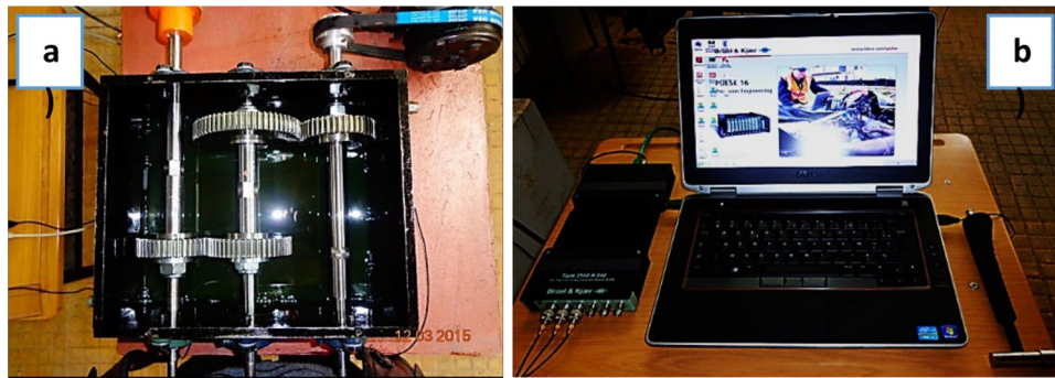
Fig. 5 (a) Experiment's test rig, (b) PULSE system for signal acquisition, post-processing, and data analysis type Brüel & Kjær 18th version with four (04) inputs and two (02) output channels. All the experiments are carried out in the following conditions: Driveshaft
