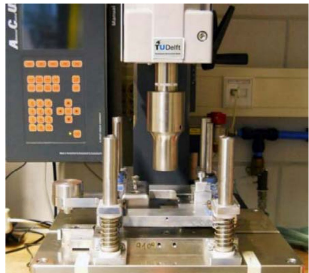
Fig. 4 The clamping device for locating and clamping laminate panels in ultrasonic welding [61]
