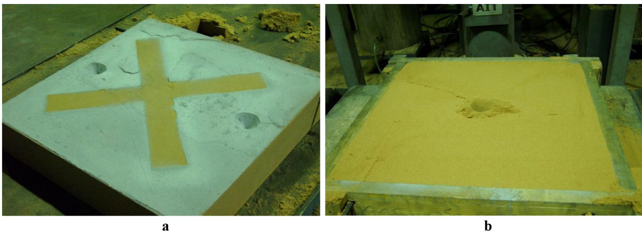
Fig. 3 Manufacturing technology: a bottom half-mold with a model; b mold prepared for pouring
