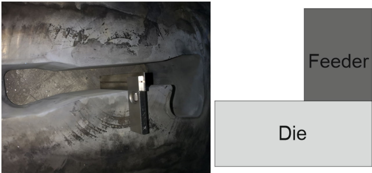
Fig. 12 Regular feeder geometry
