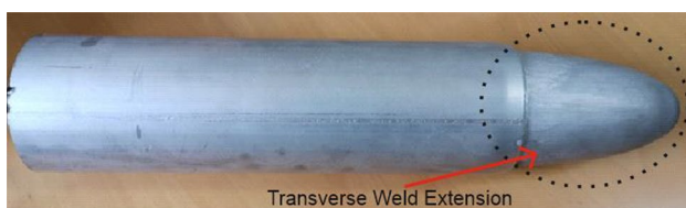
Fig. 11 Charge weld formation and transverse weld extension during the extrusion of 6082 aluminum alloy
