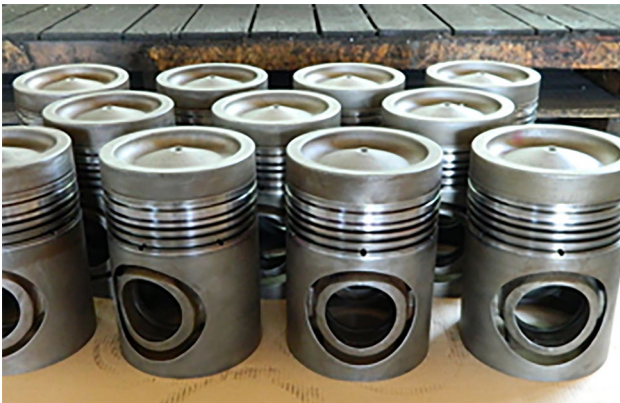
Fig. 13 MAN B&W pistons repaired with the LP-DED process
