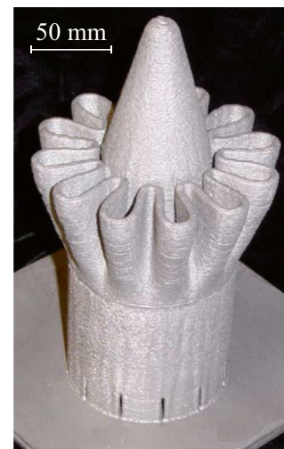
Fig. 25 Ti64 1/16 scale model of a mixing nozzle for a gas turbine produced by Bell Helicopter (courtesy of Optomec®) [195]
