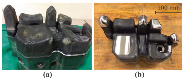
Fig. 11 a Damaged and b restored automotive die [92]
