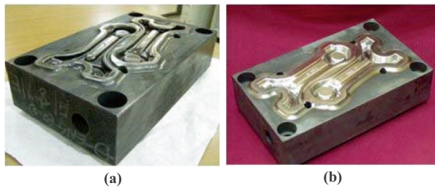
Fig. 10 a Damaged and b restored hot forging die [88]
