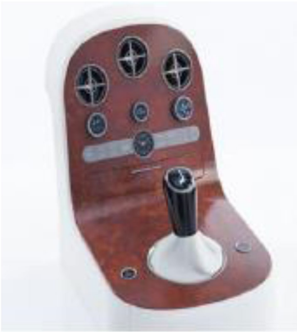
Fig. 3 Full-coloured, textured visual prototype centre console produced using AM [84]
