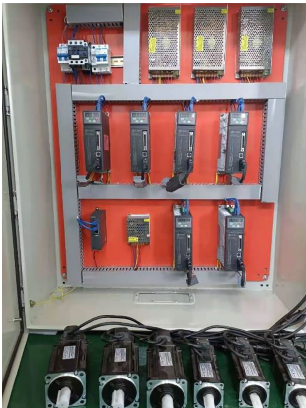
Fig. 26 Hardware platform of six-axis motion control system
