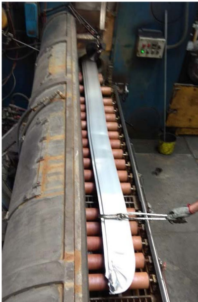
Fig. 6 The extrusion of the first billet
