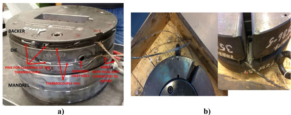
Fig. 5 The installation of the thermocouples: a in the die and backer, b outside the external ring
