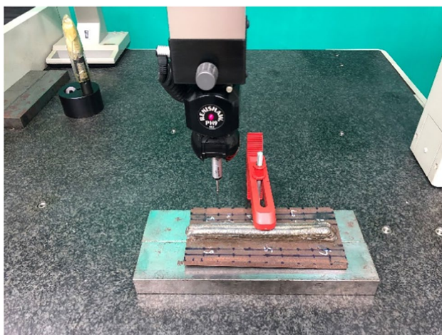
Fig. 3. Investigation of substrate deformation using CMM Mitutoyo Beyond 707
