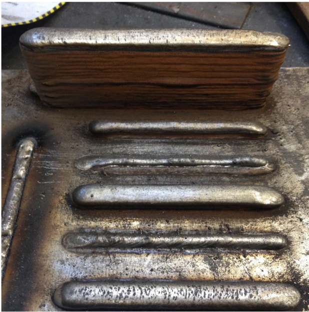
Fig. 3 Example of wall deposition using different parameters
