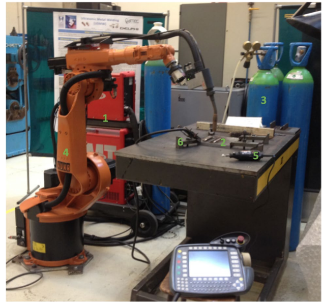
Fig. 1 Set up of the experiment: (1) Fronius VR 7000 CMT (cold metal transfer) power source; (2) substrate plates; (3) shielding gas; (4) 6-axis KUKA robot; (5) grinder; (6) jigs for clamping
