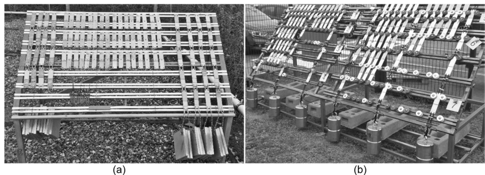
Fig. 5 Outdoor exposure of joint specimens a at the ZINQ site in Gelsenkirchen, Germany, and b at the OCAS site in Zelzate, Belgium
