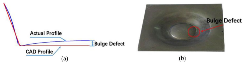
Fig. 13 The failure mode of the bulge defect. (a) Schematic of bulge defect and (b) bulge defect in actual part [48]
