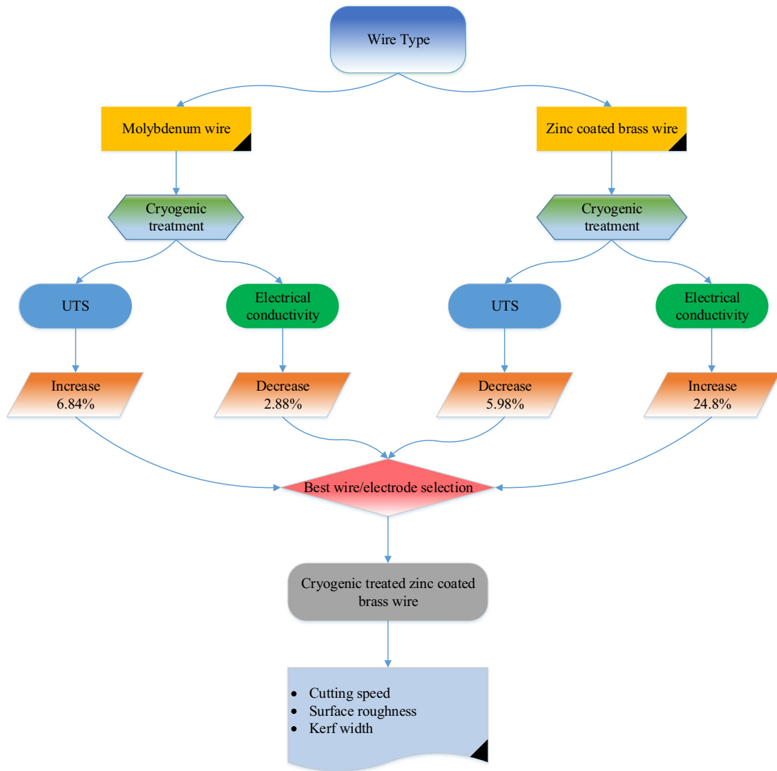
Fig. 3 Framework for the selection of appropriate wire electrode for the machining of the squeeze casted Al2024/Al 2 O 3 /W hybrid composite
