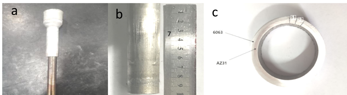
Fig. 4 a Forming billet and b extruded tube, c cross section of extruded tube
